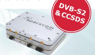
**XLink-S** is an advanced transceiver system (Software Defined Radio – SDR) for S band communication links of small satellites in LEO environment. The mechanical dimensions fit a 1U CubeSat as well as larger satellites. The radio interface and radio protocol were developed according to standard CCSDS protocols.
